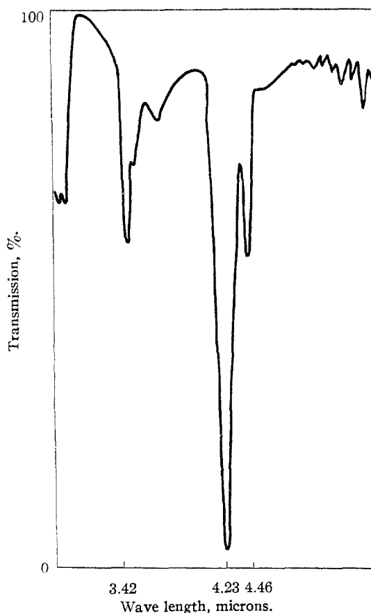
Fig. 3.—Infrared spectrum* of adiponitrile 0.0005-inch liquid cell.
